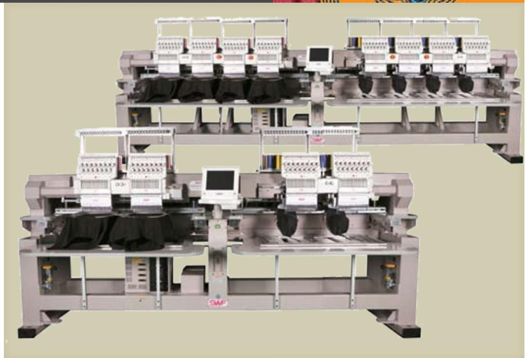
Highly productive and efficient, these machines feature exclusive patented technology that allows for embroidering two different designs simultaneously on either flat or tubular format.
